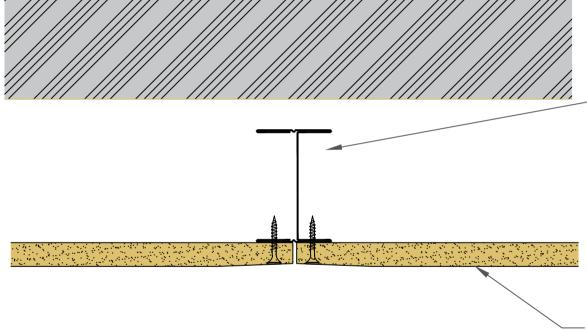
SPEEDLINE 60mm 'I' Studs at 600mm Ctrs
